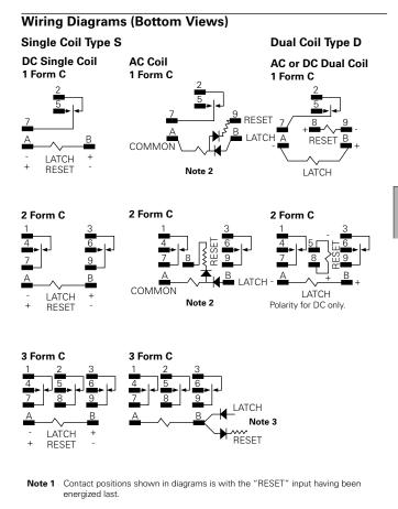
Note 2 Do not connect any low impedance loads from terminal B to A.
